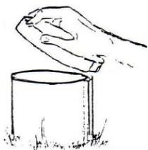
1. Remove well cap or the vent pipe or plug if the well is equipped with a sanitary well seal. Water softeners, reverse osmosis units and carbon filters may need to be on **by-pass during the chlorination and until sampling**. Manufacturers of water softeners and other water treatment devices should be contacted for specific chlorination instructions for their devices to avoid potential damage.
