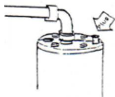
3. Connect a hose to a house spigot and run water directly into the well until **chlorine odor is present** in the water. Rinse the inside of well walls and run water this way for **15 minutes**.
